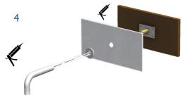
Fit Glass Splashback with adhesive (or other fixing method as required) leaving mounting assembly protruding
