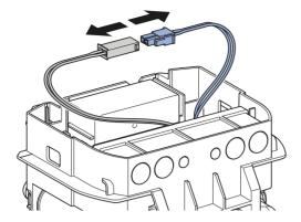
7 Remove the defective control electronics.
