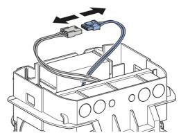
6 Disconnect the solenoid valve cable.
