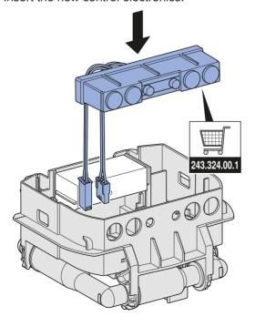
**9** Connect the cable for the solenoid valve.
