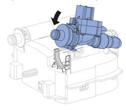
15 Connect the cable for the solenoid valve.
