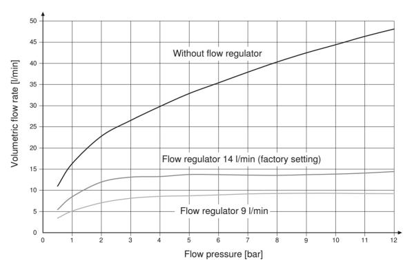
Figure 2: Characteristic curve of flow rate
