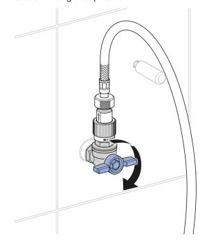
**4** Demount and dispose of the water pressure reducing valve.
