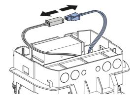
6 Remove the solenoid valve unit.
