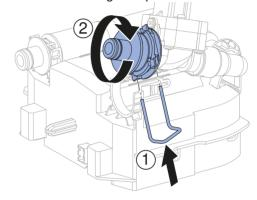
14 Snap the solenoid valve unit into place.
