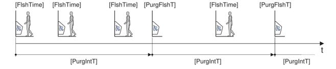
The purging flush can be used together with the interval flush or the hybrid mode.
