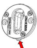
TACCA INFERIORE NOTCH FACING DOWN
