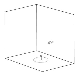
Remove the basin, install the waste pipe either at the height of the entrance horizontally, or within the perimeter of the basin vertically.
