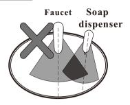
Installing electronic soap dispenser and faucetwith intersecting center lines might lead toaccidental activation of either or both.
