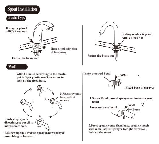
Please exercise special care not to cut the soap hose or damage sensor cable while fastening the brass nut.
