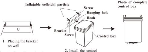
Tips: horizontally putting the bracket on wall and mark down the positions of screws' holes by pencil and then drill the holes and finally affix the bracket on wall.
