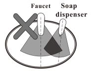
Installing electronic soap dispenser and faucetwith intersecting center lines might lead toaccidental activation of either or both.
