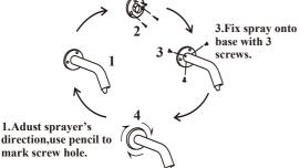
4. Screw up the cover on sprayer, now sprayer assembling in finished.
