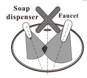
Keep sensor range adjustment within 4 inches away from center of spout. This can only be done with optional remote control.
