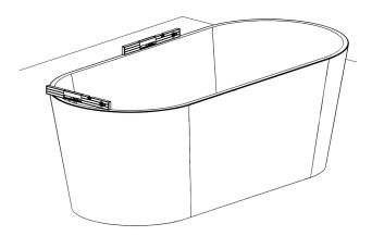
Place the bathtub onto the finished floor level. Make sure that both horizontal axis are level. Levels can be adjusted by shims (not included).
