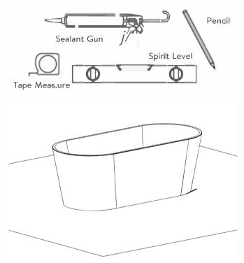
Carry the bathtub, and place in the final position, using a pencil draw around the perimeter of the base, this will help you re-align the bathtub on final fixing.
