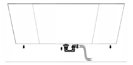
Connect the waste, remove the support and gently move the bathtub in to the position.
