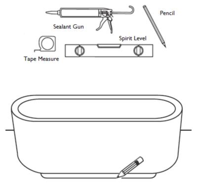
Carry the bathtub, and place in the final position, using a pencil draw around the perimeter of the base, this will help you re-align the bathtub on final fixing.
