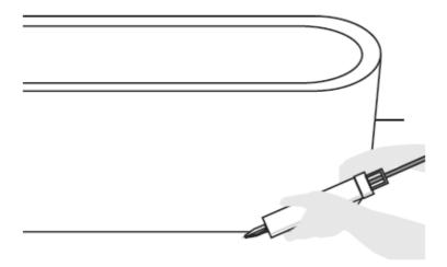
Remove the water from the bathtub, apply a bead of silicon around the outer perimeter.
