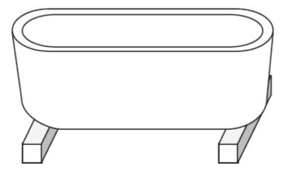
The waste can now be connected, for ease leave the bath in position but raise it by using 2 pieces of 4"x4" timber, this will give you adequate room to connect the waste.
