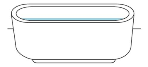
Filling the bath with water will help with the final levelling and show any further "shim" areas required.
