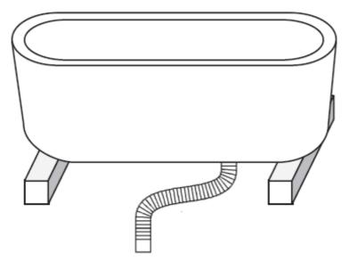
The flexible waste can be connected in 2 ways, 1. Can be connected after the bottle trap and the connected to the waste pipe under floor level. 2. Connected to the bath waste and then taken through the floor level to a trapped gully.
