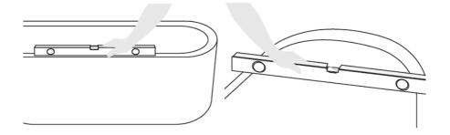
Place the bathtub onto the finished floor level. Make sure that both horizontal axis are level.
