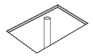
Remove the bathtub, inside the pencil line perimeter arrange the waste in the floor.
