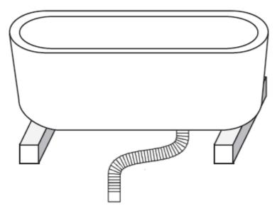
The flexible waste can be connected in 2 ways, 1. Can be connected after the bottle trap and the connected to the waste pipe under floor level. 2. Connected to the bath waste and then taken through the floor level to a trapped gully.
