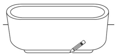
Carry the bathtub, and place in the final position, using a pencil draw around the perimeter of the base, this will help you re-align the bathtub on final fixing.
