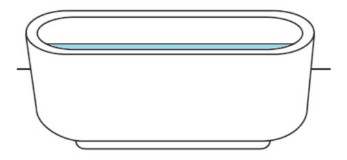
Filling the bath with water will help with the final levelling and show any further "shim" areas required.
