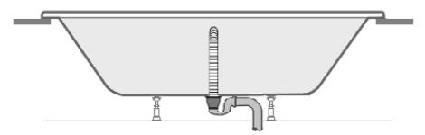
Connect the waste assembly to the bath tub, and fill with water. This will help level and bed the bath in
