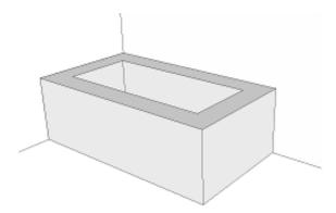
If the bath is inset, firstly measure the size of the bath and mark this on the top. Then make the opening smaller on all sides by approx. 20-30mm, this will allow the bathtub to be supported around the perimeter of the rim.
