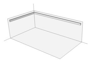
If the tub is to be installed directly against the wall, please ensure that 2 batons are secured to the wall, this will support the bottom lip of the bathtub.
