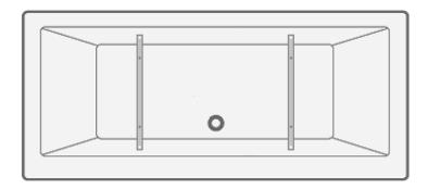
Whilst upside down, use the screws supplied with the bath leg set and secure the two bars evenly across the bath tub.
