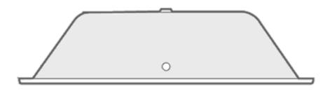
Carry the bath near to where the bath is going to be installed and turn upside down, its recommended to lay the bathtub onto a protective sheet/blanket.
