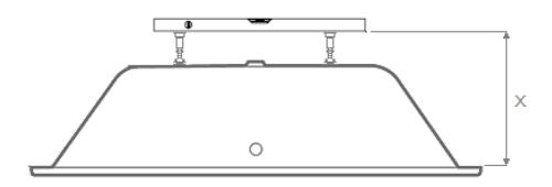
To make installation easier, firstly measure the required height the bathtub is to be inset too (X), adjust the legs to this height and level across. The bathtub is now prepared.
