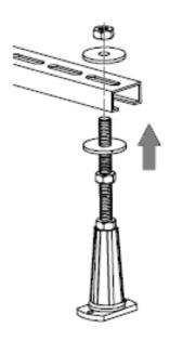
Screw the foot onto the threaded bar, screw one nut to the base, screw on a further nut and washer onto the threaded bar then push the assembly through the bar and secure with another washer then nut.
