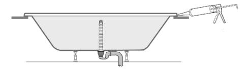
Empty the water from the bath, place a small bead of silicone around the perimeter of the bath tub
