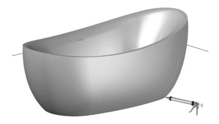
Remove the water from the bathtub. apply a bead of Silicon around the outer perimeter,
