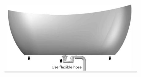
Connect the waste, remove the support and gently move the bathtub in to the position.
