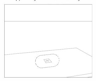
Remove the bathtub, inside the pencil line perimeter arrange the waste in the floor.
