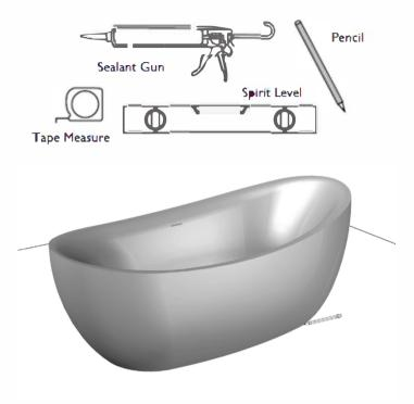
Carry the bathtub, and place in the final position, using a pencil draw around the perimeter of the base, this will help you re-align the bathtub on final fixing.
