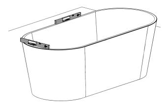
Place the bathtub onto the finished floor level. Make sure that both horizontal axis are level.
