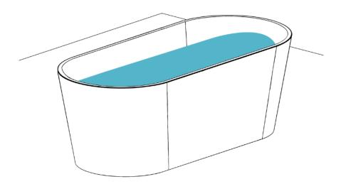
Filling the bath with water will help with the final leveling and show if any further "shim" areas required.
