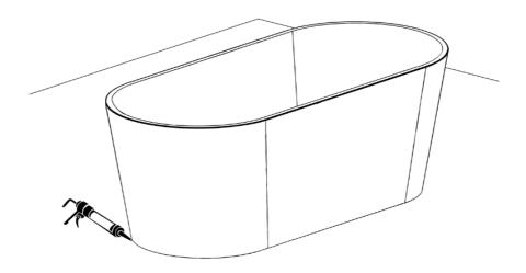
Remove the water from the bathtub. apply a bead of Silicon around the outer perimeter,
