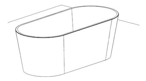
Allow the silicon to cure for up-to 8 hours, after this time has passed the installation is
