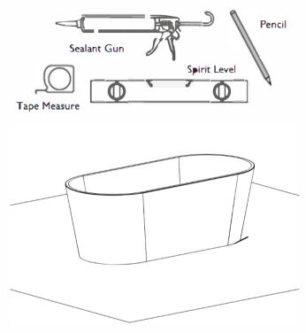
Carry the bathtub, and place in the final position, using a pencil draw around the perimeter of the base, this will help you re-align the bathtub on final fixing.
