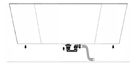
Connect the waste, remove the support and gently move the bathtub in to the position.
