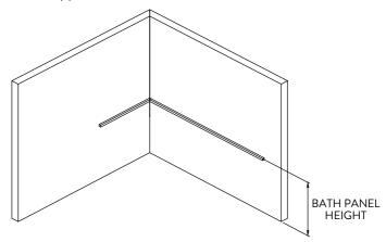
Install the bath against the wall, ensuring that the bath rests on the timber batten
