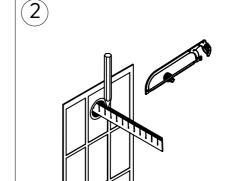
Measure the depth of the inner thread of cold & hot water pipes and mark it. This is to have NO gap left btw the wall and brass connector. Cut the extra length of the outer thread of the brass connector at marked length.
