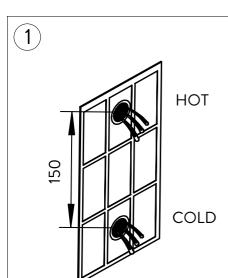
Make sure cold & hot water pipes installed at 1050mm height. Flush the pipes before installation. Make sure the middle distance btw the two pipes are 150mm, and allow 5mm adjustment.
