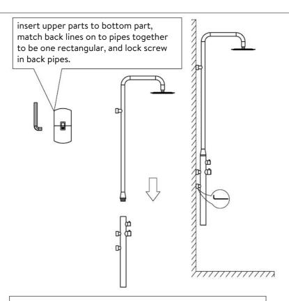
insert upper part to upper holder, lower parts to the two brass connectors, then tighten the screws. Connect the seperate shower head if have, and instal handshower and hose to hose inlet, then all installations are done.
