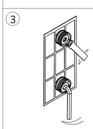
Fit the two brass connectors to the stainless fixing plate with two holes. Then tighten the two brass connectors to the cold & hot water pipes.
