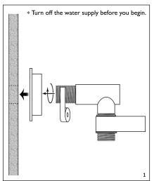
Wrap the inlet thread with PTFE tape and install in to the wall fixing. Run water through the shower outlet to flush out any dirt and debris.
