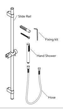
Select a convenient height to place the shower rail based on your personal needs. Mark the place for drilling the hole in wall.
