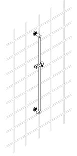
3 Install hand shower by using thread tape.
