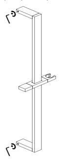
Insert anchors into drilled holes & fix posts with screws. slide the slide rail onto posts & fix slide rail with with allen key.
