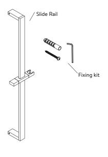
1 Select a convenient height to place the shower rail based on your personal needs. Mark the place for drilling the hole in wall.
