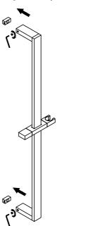
Insert anchors into drilled holes & fix posts with screws. slide the slide rail onto posts & fix slide rail with with allen key.
