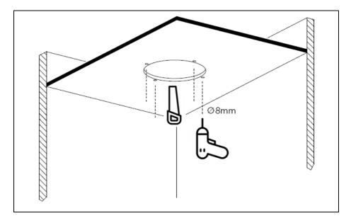
Drill the position holes and cut out the internal diameter previously marked.
