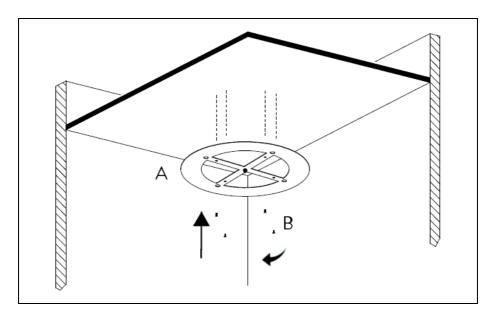
Fix the frame A to the false ceiling with 4 screws B provided.
