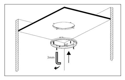
Install the cover frame by tightening the screws into the circular frame using the Allen key.  $\,$
