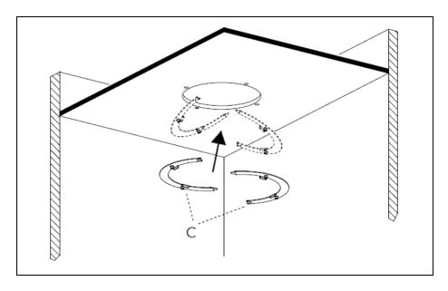
Place the circular frame C in position on top of the false ceiling
