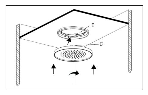
To fix the shower head, insert pins D into hook E on the frame and rotate anti-clockwise.
