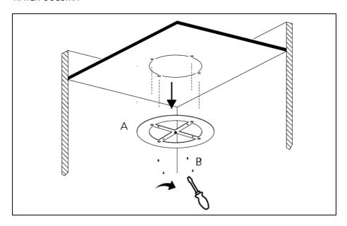
After marking with a pencil, remove the frame A from the false ceiling.
