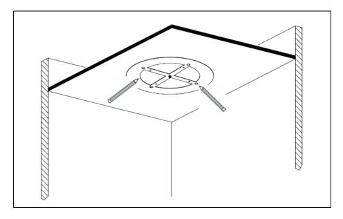
With a pencil, mark the position holes and the internal diameter of the frame.
