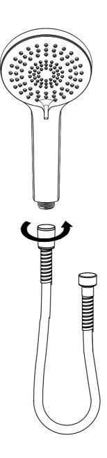
Insert the screen washer into the end of the inlet of the handshower hose. Tighten the handshower onto the hose until hand tight. Do not over tighten.
