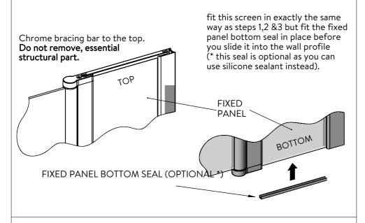
4. Fit screen bath seal to glass panel and silicone as below - - - - allow 24 hours to dry before using.
