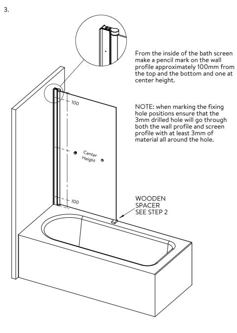
Fit the small screws, cup washer and chrome cap in 3 positions. The screen is now fixed in place
