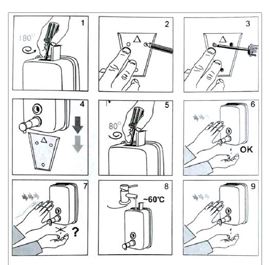
Filled with liquid soap below the MAX line level. The back wall must not be flooded with soap, if it happens it is recommended to dismount and wash it thoroughly.
