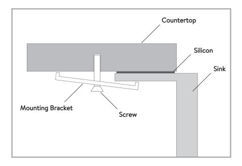
6. Apply a bead of silicon sealant at the edge of the sink fill any gap. Wipe away any excess silicon and allow to dry.
