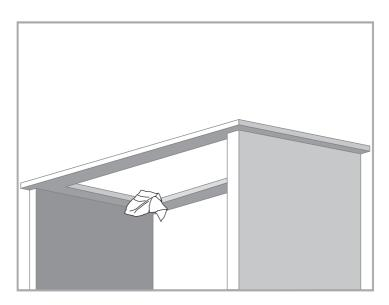
3. Loosely attach the mounting brackets to the underside of the counter top.
