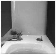
1. Insert the screw on the hinge base into the holes on the pan.
