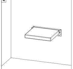
Fasten the PU seat pad on the bracket by 2 pcs screws and ensure the seat pad can be moved along guide channel smoothly, then these screws can be locked.
