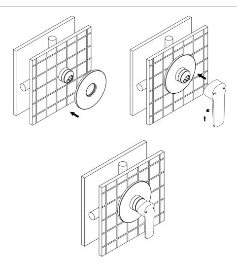
Once the surrounding finishes have been applied (Tiles/Marble etc.) remove the protection covers. Fit the face plate onto the mixer body, it is advised to use a small amount of lubricant on the rubber seals. Slide the handle onto the cartridge pin and secure with the grub screw, then push on the cover cap.
