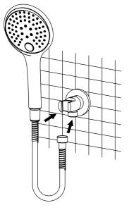
Install the hose onto the shower outlet. Use a suitable spanner to tighten the hose onto the shower outlet. Do not overtighten. Insert the screen washer into the end of the inlet of the handshower hose. Tighten the handshower onto the hose until hand tight. Do not over tighten.
