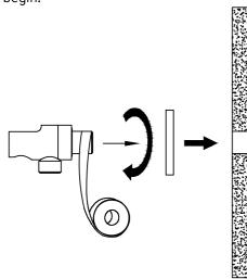
Wrap the inlet thread with PTFE tape and install in to the wall fixing. Run water through the shower outlet to flush out any dirt and debris.
