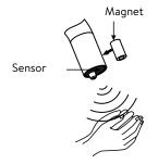
Approach the magnet to the sensor at the top of the faucet, the led light will flash continuously, then place your hand/object at the appropriate position as reference, take away your hand/object when the led light is off. The sensor adjustment is finished.
