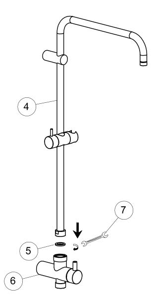
1. The G3/4"joint of the water inlet end of the shower pipe (4) is fitted with a sealing gasket (5) and inserted directly into the water separator (6), and is fixed by a wrench (7)
