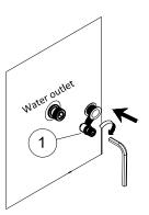
2. Insert the intake joint into the water separator (2), keep the top and bottom joint of the water separator vertically parallel, lock the top screw (3) with the hexagon wrench and tighten it.
