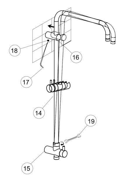
4. After the wall seat is installed, the shower tube (14) is reinserted back into the water separator (15), and then the fixed seat (16) is sheathed into the fixed wall seat mounted on the wall in the reverse direction of the arrow head, and the top screw (18) is tightened with a hexagon wrench (17), finally, use a wrench (19) to tighten the connection between the pipe and the water separator.
