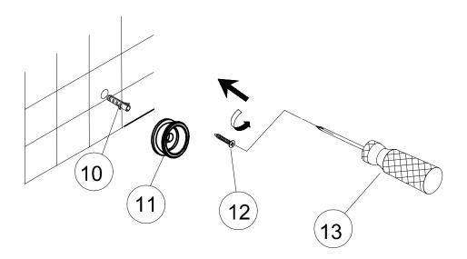
3. The expansion sleeve (10) is inserted into the hole according to the position of the hole of the fixing seat (11) drawn by a pencil, the fixing seat is installed on the wall with a self-tapping screw (12), and the screw is tightened with a screwdriver (13).
