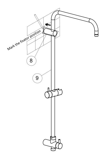
2. Position the shower tube (9) fixing seat assemble (8) close to the wall, mark the fixing seat diameter with a pencil, and remove the shower tube.
