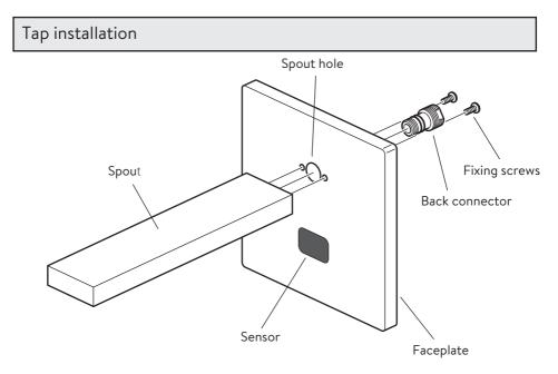
For ease of installation the faceplate and battery can be disconnected from the unit at the connectors.
