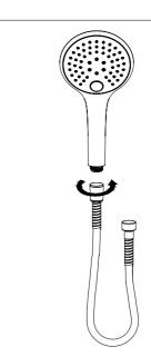
Insert the screen washer into the end of the inlet of the handshower hose. Tighten the handshower onto the hose until hand tight. Do not over tighten.
