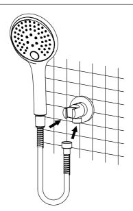
Install the hose onto the shower outlet. Use a suitable spanner to tighten the hose onto the shower outlet. Do not overtighten.
