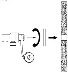
Wrap the inlet thread with PTFE tape and install in to the wall fixing. Run water through the shower outlet to flush out any dirt and debris.
