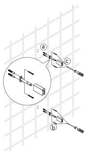
Slide the slide rail onto post (don't use to much force). Insert covers on both slide rail ends.
