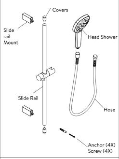
1 Select a convenient height to place the shower rail based on your personal needs. Mark the place for drilling the 4 hole in wall.
