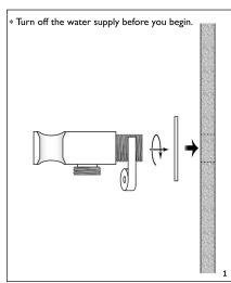
Wrap the inlet thread with PTFE tape and install in to the wall fixing. Run water through the shower outlet to flush out any dirt and debris.
