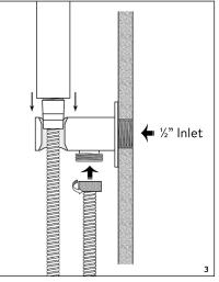
Install the hose onto the shower outlet. Use a suitable spanner to tighten the hose onto the shower outlet. Do not overtighten.
