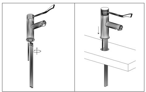
Install the threaded rods and **hand**-tighten the pipes into the bottom of the mixer body.
