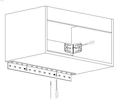
Gently lift the cabinet into position and place on the support bracket. Make sure that the cabinet is securely held in place before letting go. When you are happy with the position of the cabinet, using wall fixings, fix the cabinet through the angle brackets at the rear of the unit, and then secure the vanity to the support bar fixing screws from the bottom vanity.
