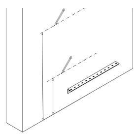
Once you have decided on a suitable position for your vanity unit, measure 850-900 from finished floor level, mark out the drilling positions on the wall. Then measure the distance between the fixing holes to the bottom of the vanity. Use this measurement to draw a horizontal line across to fix the support bracket.
