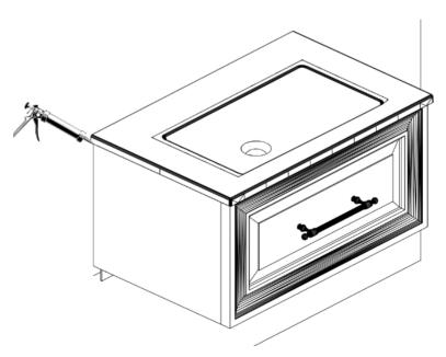
Install basin as per the basin installation, to finish please a bead of silicon around the top perimeter of the basin.
