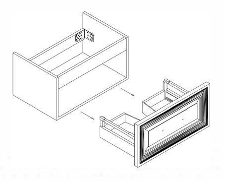
To make installation easier it is recommended that you remove the drawer from the cabinet. Pull the drawer out, with both hands at each side of the drawer reach under the base of the drawer sides at the front and feel for the release mechanisms.
