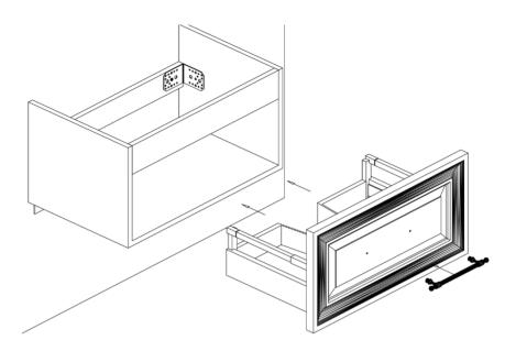
Put the drawer back into the unit. Fully extend the drawer runners and lower the drawer onto the runner pushing it closed, the drawer will click into place. Then fix the handles (Not included).
