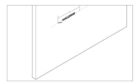
Once you decided on a suitable position for your Countertop, mark out the external distance on to the wall (X). Line the wall brackets up to the inside of the markings and mark out the drilling positions on the wall.
