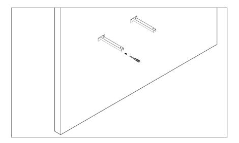
Attach the brackets on the wall using suitable fixings (Not supplied). Making sure the brackets are level and the distance between the outer edges of the brackets are the same as the measure (X) in the previous stage.
