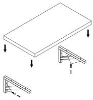
Once you have decided on a suitable position for your countertop, mark out the external distance onto the wall. Then measure the center of the distance and mark, Half the dimension and mark this distance either side of the center line. Position the brackets and mark the fixing holes.
