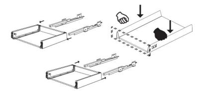
Put the drawer back into the unit. Fully extend the drawer runners and lower the drawer onto the runner pushing it closed, the drawer will click into place.
