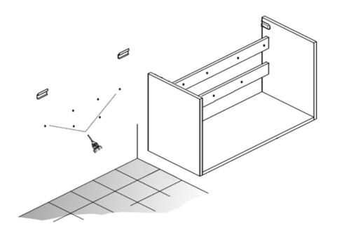
Carefully remove the cabinet, drill and plug the markings for the rear support bars.
