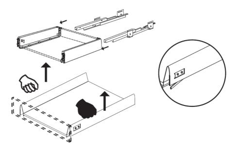
To make installation easier it is recommended that you remove the drawer from the cabinet. Pull the drawer out, with both hands at each side of the drawer reach under the base of the drawer sides at the front and feel for the release mechanisms. Push the plastic clips inwards and at the same time lift the drawer unit up clear of the runners.
