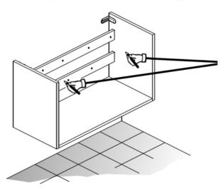
Gently lift the cabinet into position so that the cabinet hangers sit onto the wall brackets. make sure the unit is level and adjust if required. Mark the 6 holes on the rear support bars.
