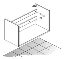
When you are happy with the position of the cabinet, using suitable wall fixings (not supplied), fix the cabinet through the rear support bar.
