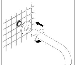
Fix the filter, clean and replace the filters regularly to make sure the spout work properly and durability.
