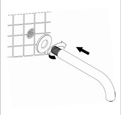
Fix the filter, clean and replace the filters regularly to make sure the spout work properly and durability.
