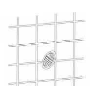
Clean carefully the pipes and check the water flow before connecting the tap to the system to ensure a good operation.
