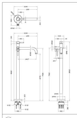
2 The concealed base needs to be installed onto the stable substrate 55mm (min) from finished floor level. The water supply pipes will also need to be positioned under the finished floor level.
