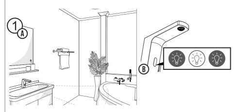
Automatically setting the initial value of the sensing distance: The sensor first scans the use environment 8 times with power on to set the sensing distance.
