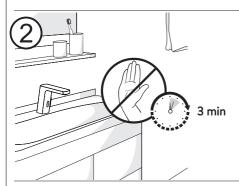
After setting the initial value of the sensing distance, the sensor should be not used for 3 minutes. During this period, the sensor repeatedly scans the use environment, and then automatically sets the optimal sensing distance according to the scan parameters.
