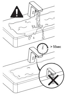
Timeout protection: when the continuous use time exceeds 55' seconds, the sensor will automatically turn off the water, so as to avoid the phenomenon of continuous water flow caused by foreign objects in the sensor' range and waste of water.
