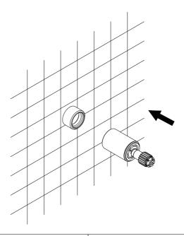
3 Slide the cover plate on to the cartridge against the wall and put handle on cartridge pin and secure with elan key.
