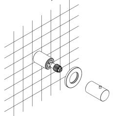
4 Open the water supply and retest for leaks.
