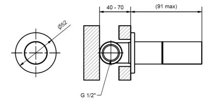
1 Install the stop valve into wall and connect the inlet and outlet water supplies, please test to check any Leaks.
