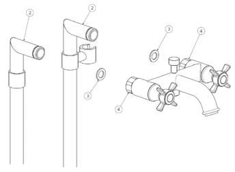
Insert the gaskets (3) into the nuts (4).
