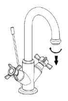
Periodically the aerator will need to be cleaned, simply unscrew the aerator housing
