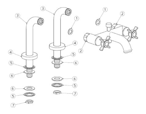
Cold water inlet on the right, hot water inlet on the left.
