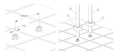
Cold water inlet on the right, hot water inlet on the left.
