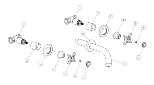
When the wall covering is applied, remove the protection caps and hand tighten the cover (2), insert the rosette (3), hand tighten the cap (4) and assemble the handle (5), secure it by tightening the screw (6).
