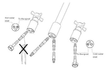
Hand tighten the flexible hoses as shown in the picture.
