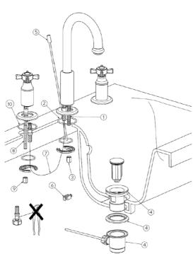
Hand tighten the threaded shaft (1) on the spout and insert the gasket (2) between the spout and the basin.
