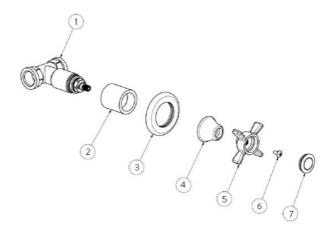
When the wall covering is applied, remove the protection caps and hand tighten the cover (2), insert the rosette (3), hand tighten the cap (4) and assemble the handle (5), secure it by tightening the screw (6). Hand-tighten the cap (7).
