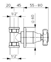
Prepare a suitable hole in the wall and insert the rough parts (1) with the protections on (dimensions mean at finished wall including the coating). Make connections (cold water right / hot water left).
