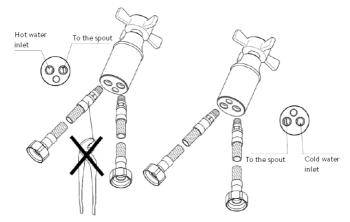
Hand tighten the flexible hoses as shown in the picture.
