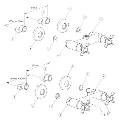
Cold water inlet on the right, hot water inlet on the left.
