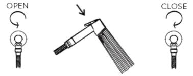
Open the angle valve, test the bidet spray by pushing down on the button/lever to make sure then water comes through evenly, close the angle valve after use.
