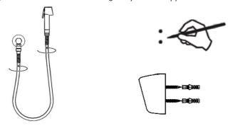
Hand-tighten the flexible hose onto the bidet-spray and to the water supply angle valve, place the bracket to wall at the correct height so that hose does not touch the floor and is within the length of the hose, mark, drill and secure to the wall.
