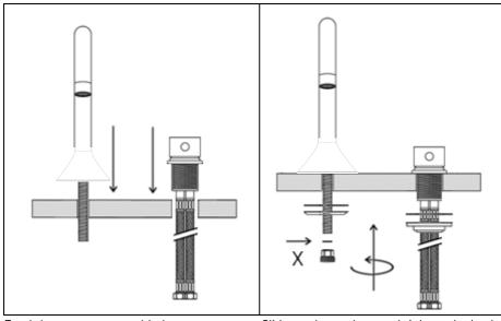
Feed the two pre-assembled components through the holes in the basin/countertop.
