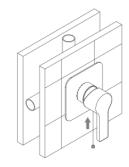
Once the surrounding finishes have been applied (Tiles/Marble etc.) remove the protection covers. Fit the face plate onto the mixer body, it is advised to use a small amount of lubricant on the rubber seals. Slide the handle onto the cartridge pin and secure with the grub screw, then push on the cover cap.
