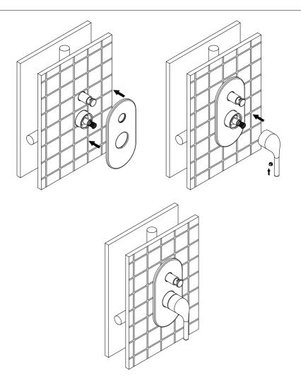
Once the surrounding finishes have been applied (Tiles/Marble etc.) remove the protection covers. Fit the face plate onto the mixer body, it is advised to use a small amount of lubricant on the rubber seals. Slide the handle onto the cartridge pin and secure with the grub screw, then push on the cover cap. Open the water supplies and re-test for leaks.
