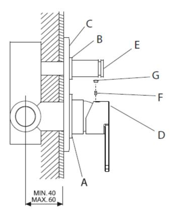
Install the mixer housing (A) at a depth so that the finished surface is between the Min/Max distance markings shown in the diagram.
