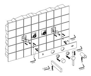
Install the spout extension and the hand-shower holder, secure with the screws provided. Screw on the cover shroud to the mixer body. Fit the face plate onto the mixer body and spout extensions, it is advised to use a small amount of lubricant on the rubber seals. Install the spout onto the extension and secure with the 2x grub screws, do the same for the hand-shower holder. Push the handle onto the cartridge pin and secure with the grub
