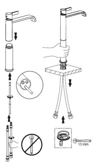
Place the threaded rod and 2 flexible pipes into the body of the mixer, place the assembly over the extension piece and through the basin / counter, From the underside, place the 'O' ring followed by the metal 'C' washer onto the threaded rod, then tighten to clamp the mixer to the basin / counter with the back nut, being careful not to over tighten.
