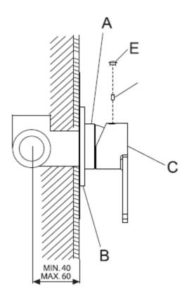
Install the mixer housing (A) at a depth so that the finished surface is between the Min/Max distance markings shown in the diagram.
