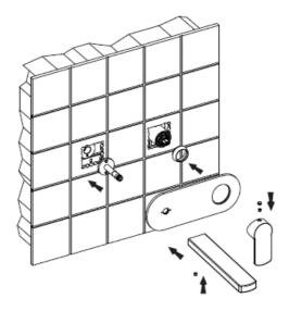
Install the spout extension and secure with the bolts provided. Screw on the cover shroud to the mixer body.
