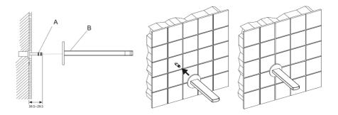
Install the spout connector (A) at the depth advised on the diagram above. Push the spout onto the connector and secure with the grub screw on the underside.
