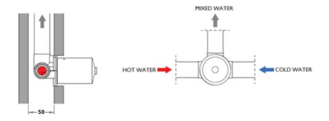
Install the mixer housing at a depth so that the finished surface is no further than the maximum distance marking shown in the diagram.
