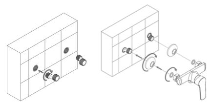
Pre install 2x ½" female fittings into the wall, these fittings should be flush to the finished wall surface. Wrap the 2 eccentrics with PTFE tape and install into the wall provisions, making sure the eccentrics are level and are the correct distance apart. Screw on the cover shrouds until secure against the wall surface.
