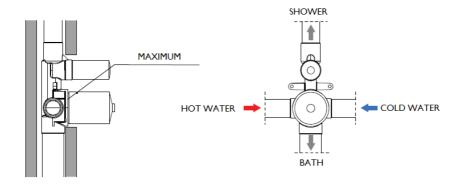
Install the mixer housing at a depth so that the finished surface is no further than the maximum distance marking shown in the diagram.
