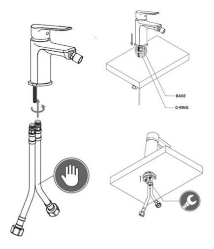
Place the threaded rod and 2 flexible pipes into the body of the mixer. place the assembly through the basin / counter making sure to install the base ring and washer.
