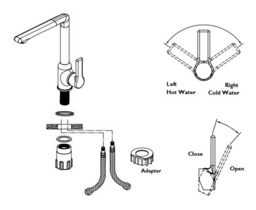
Place the 2 flexible pipes into the body of the mixer. place the assembly through the sink / counter making sure to install the base ring and washer.
